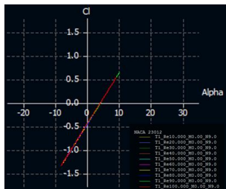
Figure C. 3 – NACA 23012 (C-130 horizontal tail) inverted aerofoil lift coefficient versus AOA (XFLR5) [38].
