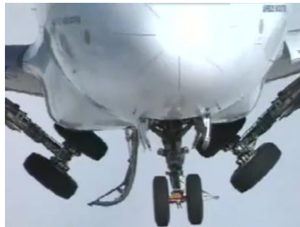
Figure 10 - Airbus A320 landing gear retraction after take-off.
