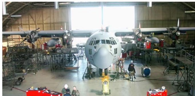
Figure 13 - Lockheed Hercules C-130 supported on jacks.
